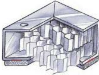
fig. 5 - Cross-cell honeycomb vent
